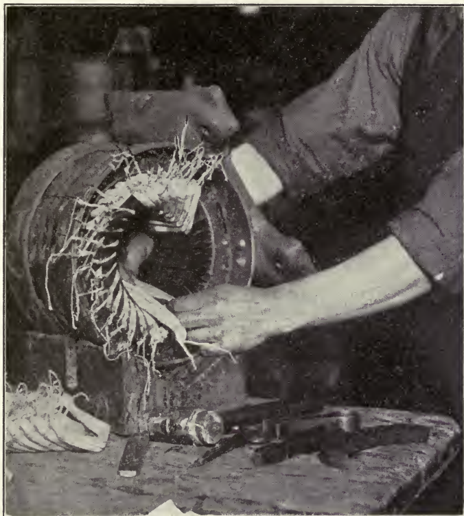
FIG. 141.—In this illustration the armature winder is shown inserting the turns of a basket coil into partially closed slots of a small induction motor stator ( Westinghouse Electric & Mfg. Company ).
